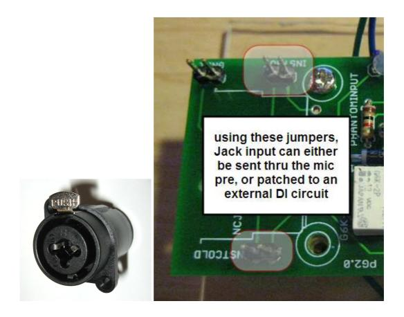
The additional GND jumper on the front on the PCB also allows the user to decide if they want to connect the connector shield into their analog ground in their system. Some users may want to experiment with this.
